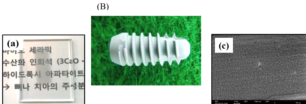
Figure1. Photography of (a) transparent HA film deposited on the glass substrate, (b) titanium implant fixture with thick HA films of more than 10 μm, and (c) SEM surface image of (b) implant fixture
